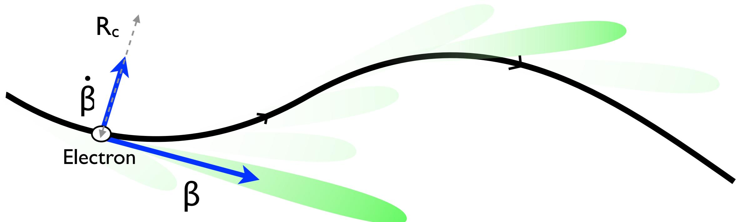
To efficiently produce X-ray radiation we need relativistic electrons undergoing oscillations
