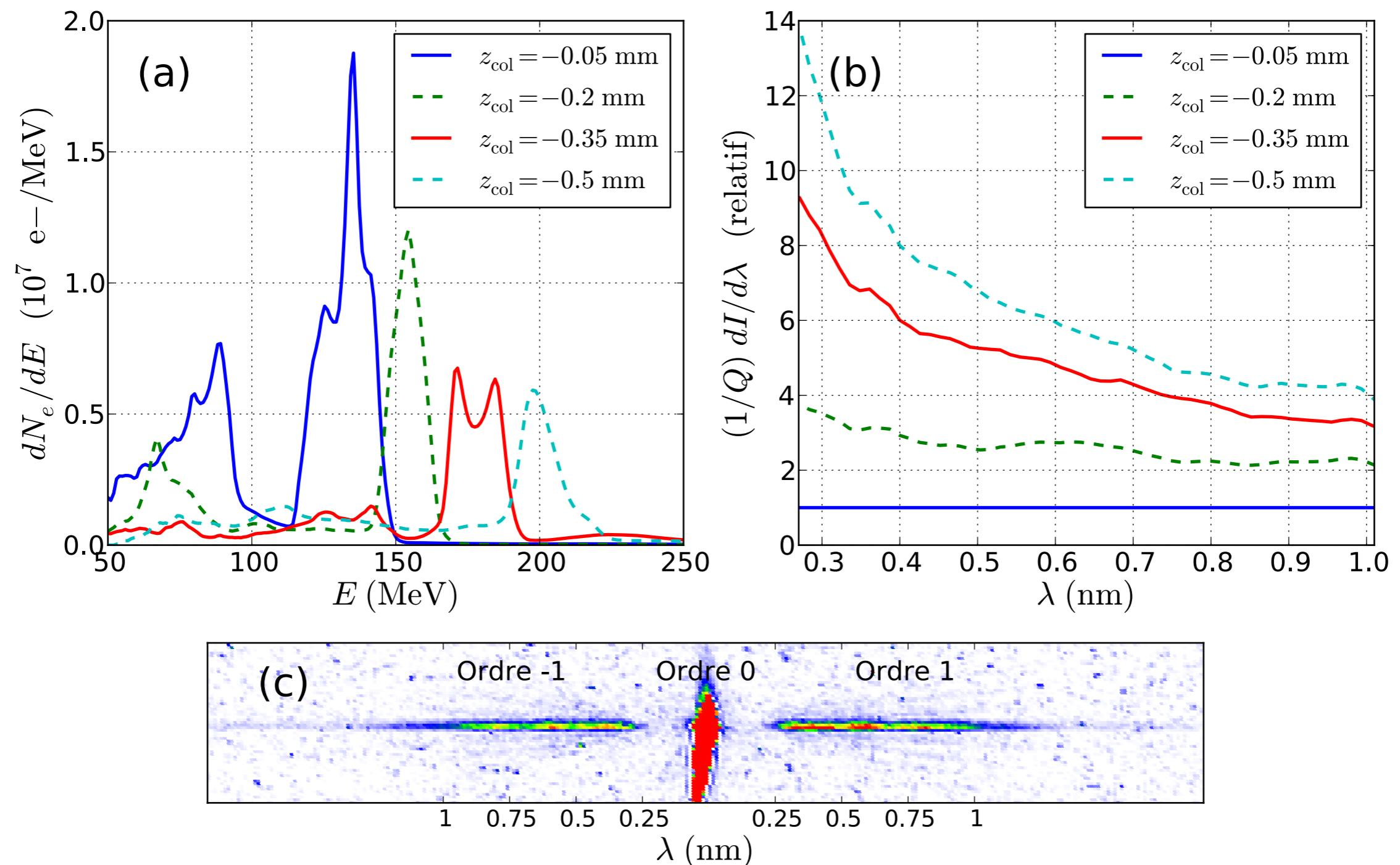
Thanks to the colliding laser pulses scheme, clear correlations between electron beam energy and betatron X ray distribution are observed
